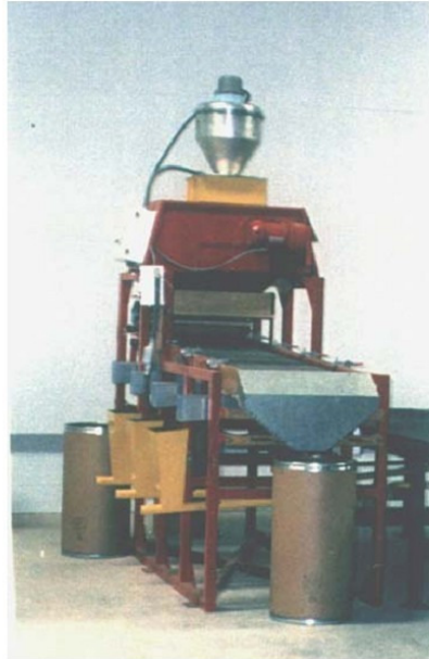
Figure 20--The SouthPine Model-156 Flat Screen Cleaner/sizer. It employs up to 5 screens to make as many as 6 size separations.
