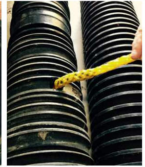
Fig. 5 Hole drilled in 1G pot which enables weekly extraction of sachet.
