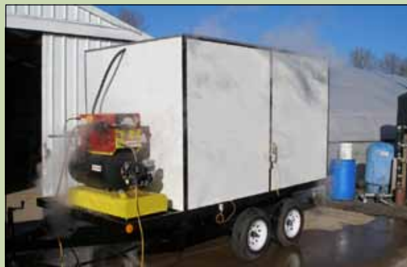
Fig. 7.2.1.f — Mobile steam pasteurization unit for small volume growers.
